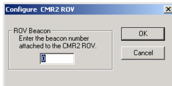
The x,y,z coordinates from the USBL are included as part of the data string output from WinFrog to the ROV. You must enter the number of the USBL beacon currently being used to track the ROV in order for WinFrog to output the desired x,y,z coordinates to the ROV. If you switch beacons during ROV operations, the beacon number must be changed in this dialog box as well.
